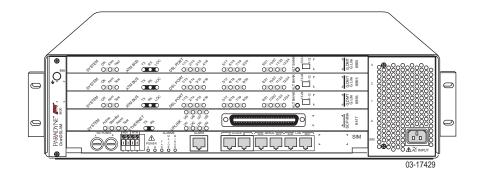
The Hotwire 8620 GranDSLAM is a 4-slot chassis designed to house one of the following combinations:
